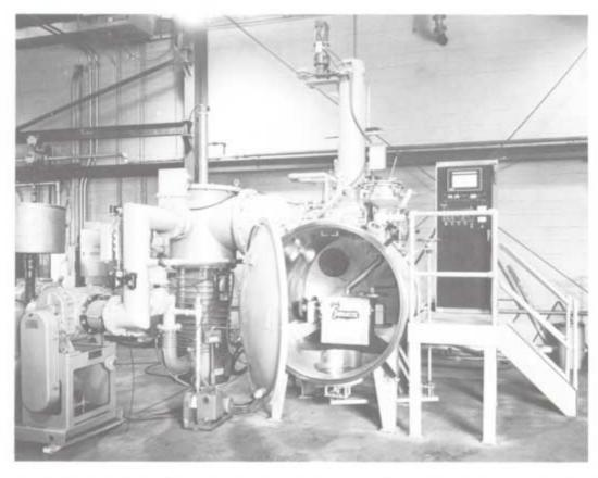
100 lb. (45 kg) vacuum induction melting furnace equipped with thermocouple probe, pyrometer sight tube, six cup additions maker, bulk charger. Interior equipped with box type induction melting furnace, tilt mechanism, baffled pumping port, multiple mold turntable, lighting. Chamber interior is stainless steel with carbon steel jacket. Control cabinet contains graphic display of pumping system, semi-automatic controls, recorder and vacuum gauging.
