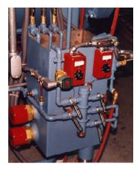
Photograph of open drain system with hot water option.
